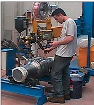
SAW robots welding of a 8" (200 mm) Class 600 valve.
