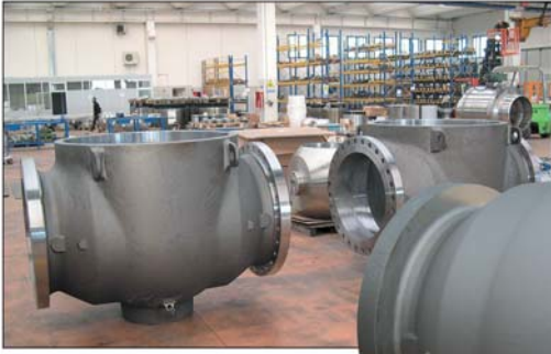
32" (800 mm) Class 300 Top-entry cast bodies in production.
