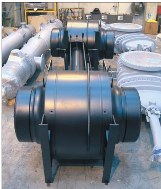
Fully welded 42" (1050 mm) Class 600 for underground service.
