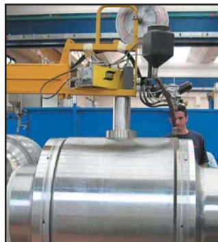
SAW robots welding of a 36" (900 mm) Class 600 valve.
