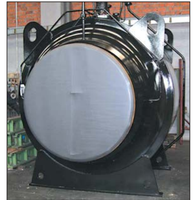
Fully welded 48" (1200 mm) Class 600 for underground service.
