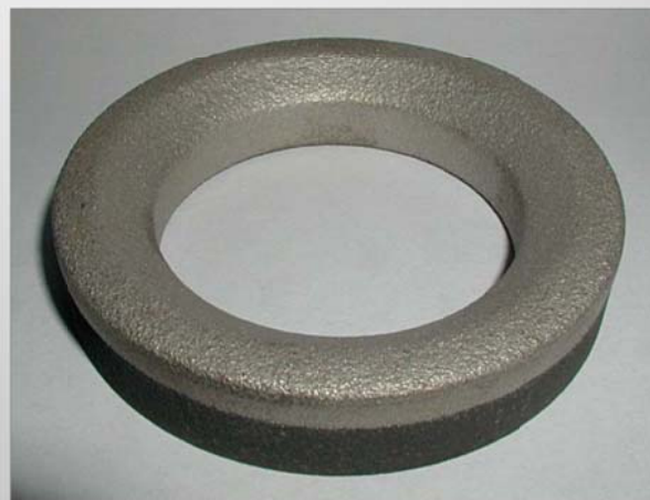
pre machined seat ring DN 2" after coating with Perrit 01
