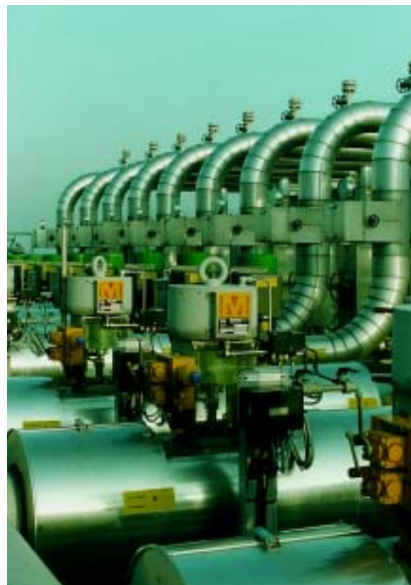
flowline shut-off valves gas production plant, N/E Netherlands (by courtesy of NAM)
