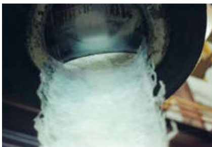
After years of use in a tough polymer application, this valve was returned to MOGAS Service facility for maintenance. Minimal repair was required before being re-installed.
