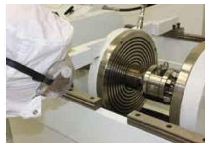
Emissions testing using clean, dry nitrogen or helium is used to shell test and seat leak test the valve in both directions, when appropriate.
