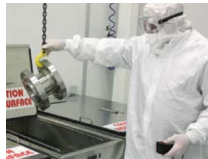
Precision cleaning—such as oxygen, aqueous and ultrasonic cleaning—of valves and critical parts reduce non-volatile residue to acceptable ISO standards.
