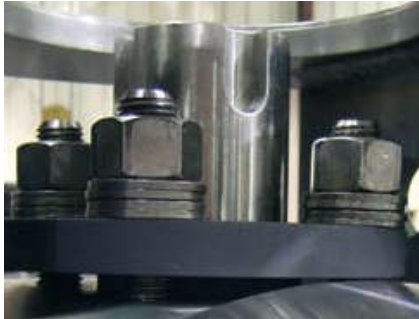
Live-loading maintains proper pressures on application-specific stem packing and anti-extrusion rings.
