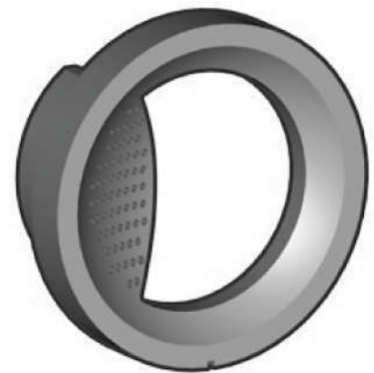
FlexStream technology uses a varying number of passageways engineered within the bore, custom designed to suit high pressure differential applications, providing better control of velocity / noise / vibration / erosion / cavitation.
