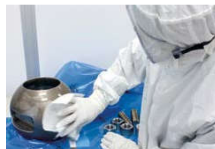
Stringent cleanroom processes for oxygen cleaning will effectively prepare parts for an oxygen-enriched environment.
