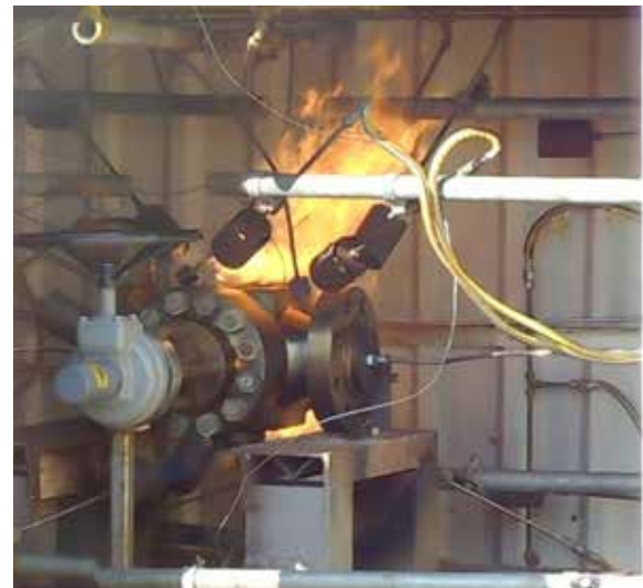
Fire safe testing of 4" - 1500 lbs
