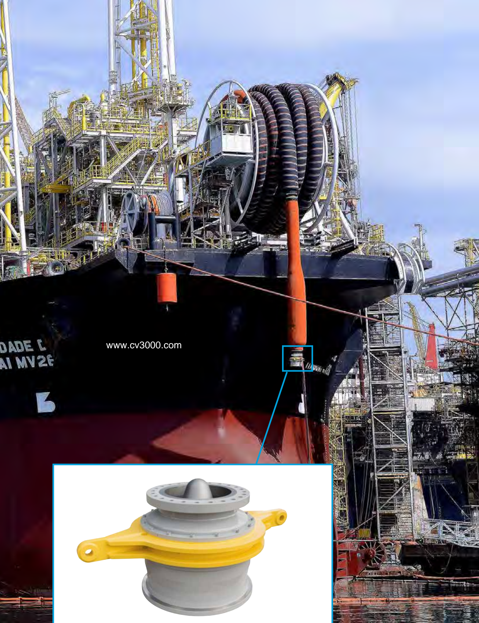
OHTP (Offloading Hose Termination Piece) for FPSO'S (in cooperation with royal IHC)
