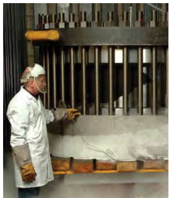
70" 150# Dual Plate Check Valve on Cryogenic Test
