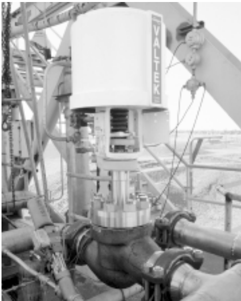
This cryogenic Mark One is used for aerospace testing as an O 2 vent valve.
