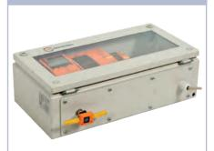
AT Mastersystems provide the Gateway to higher bus systems like Profibus or Ethernet. The "Black Box" contains all necessary components for the operation of one or two AS-i Networks. The master controls the data transfer to the Sensor-/ Actuator level while the controller processes the bus data in the integrated processor (Preprocessing of signals).
