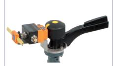
The AS-i bus connection for manual operated valves is achieved by a double sensor equipped with a flat cable connector and two inductive sensors. A puk indicates the valve position.
