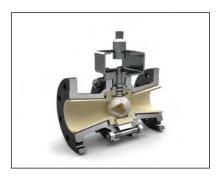
**KSV** The CeraValve type KSV is a ceramic lined ball valve for On/Off function as well as for Throttling Control applications for corrosive media with abrasive solids content. It is an alternative to PTFE/PFA lined valves in the event that their performance limits (pressure, temperature, wear) are exceeded.
