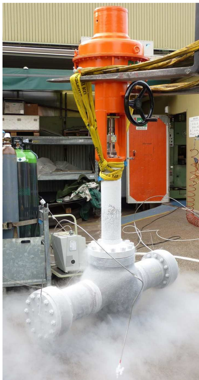
VEGA CRYO CONTROL VALVE AFTER TYPE TEST ON LIQUID NITROGEN
