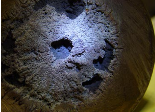
Figure 3: Cavitation damage on plug.
