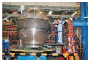
为天然气管道关键设备国产化研制的 56", Class900高压大口径全焊接球阀 56" 900# fully welded ball valve made for home-made project of key equipments on natural gas pipeline
