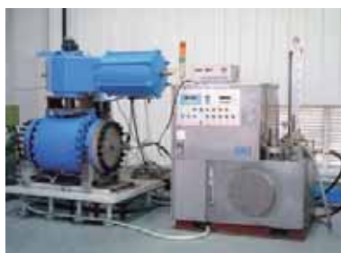
阀门寿命试验台 Valve lifetime test rack
