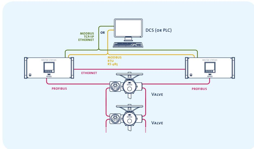
**MS202 – System and Line redundancy.** Two 19" racks featuring line redundancy. In this configuration, if the first unit is out of service, the second one ensures proper communication with the entire network. Two MS, a redundant line, up to 3 starts of lines.
