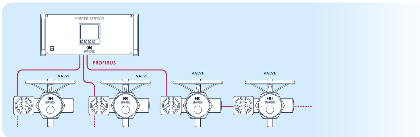
Fieldbus is interesting because it allows getting more information while reducing the overall cost of wiring and commissioning on site. Our Master Station goes further and optimizes the cable length needed to connect your actuators thanks to the **possibility to have 1 to 3 different starts of lines**. Such advantage is especially appreciated if you have 2 or 3 groups of actuators located in opposite directions, and makes you save time and resources.
