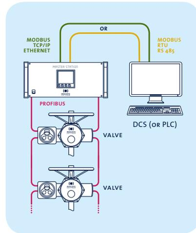
**MS102 – Line redundancy for improved reliability.** One 19" rack plus a second cable for line redundancy: more security in case of default of one cable. A single MS, a redundant line, up to 3 starts of lines.
